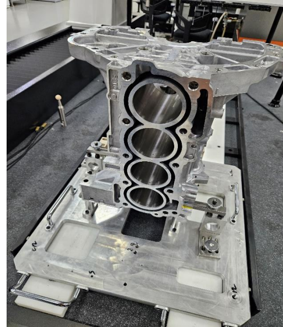
COMPONENT – HOR. BLOCK MARUTI FIXTURE PLATE FLATNESS < 20 MICRONS SIZE (520X500 MM)
