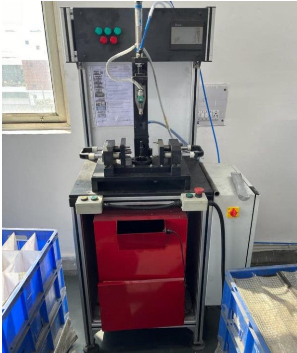
Gauging Station – Indrani CD checking & Height Measurement
