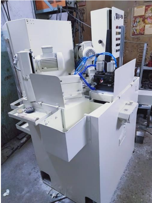
Drilling SPM: Con Rod Customer: Musashi Auto parts
