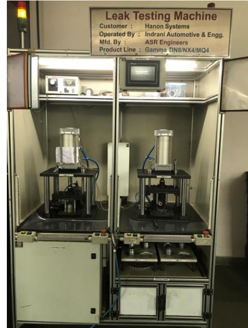
Leak Test M/C: Outlet Pipe (3models) Customer: Indrani Automotives
